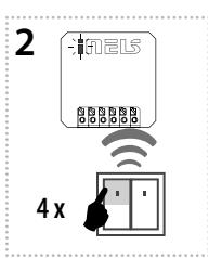
Four presses of your selected button on the RF transmitter assigns the function impulse relay (must be a lapse of 1s between individual presses).
