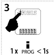
Press of programming button on receiver RFSAI-62B shorter than 1 second will finish programming mode. The LED lights up according to the pre-set memory function.
