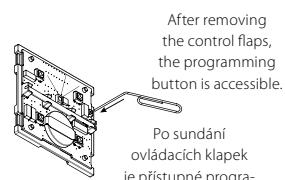
After removing the control flaps, the programming button is accessible.
