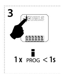
Press of programming button on receiver RFSAI-62B shorter than 1 second will finish programming mode. The LED lights up according to the pre-set memory function.
