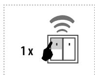
The output contact will be switched to the opposite position by each press of the button. If the contact was closed, it will be opened and vice versa.
