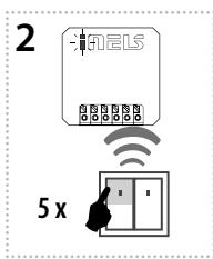
Assignment of the delayed off function is performed by five presses of the selected button on the RF transmitter (must be a lapse of 1s between individual presses).
