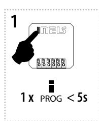
Press of programming button on receiver RFSAI-62B for 3-5 s (RFSAI-61B-SL: press for more than 1 s) will activate receiver RFSAI-62B into programming mode. LED is flashing in 1s interval.
