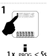
Press of programming button on receiver RFSAI-62B for 3-5 s (RFSAI-11B-SL: press for more than 1s) will activate receiver RFSAI-62B into programming mode. LED is flashing in 1s interval.
