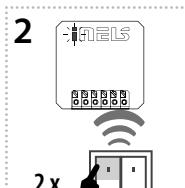
Two presses of your selected button on the RF transmitter assigns the function switch on (must be a lapse of 1s between individual presses).
